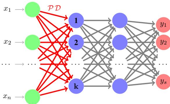
Figure 5: Fully-connected network with randomized input layer (red edges correspond to structured matrix).  $k < n$ .  $D$  is a random diagonal matrix with diagonal entries chosen independently from the binary set  $\{-1, 1\}$ , each value being chosen with probability  $\frac{1}{2}$ , and  $\mathcal{P}$  is a structured matrix. The figure should be viewed in color.
